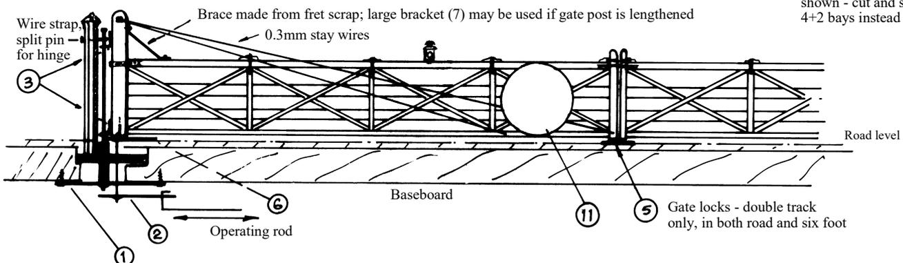
Large gate typical of a skew crossing shown - cut and shut the gates to give 4+2 bays instead of 3+3
