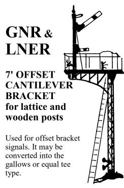
Note: this pack contains a bracket and platform only. For a complete signal, you will need: arms (S003/3 lower quadrant or S0012 series upper quadrant); a base post (S0040); dolls (S0041 or S0033 series); ladders (S009 series); finials (SC0021); and lamps (SC0026 LQ or 25 UQ).
