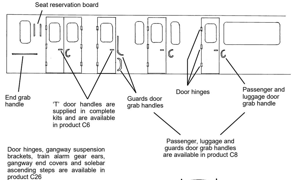
Door hinges, gangway suspension brackets, train alarm gear ears, gangway end covers and solebar ascending steps are available in product C26
