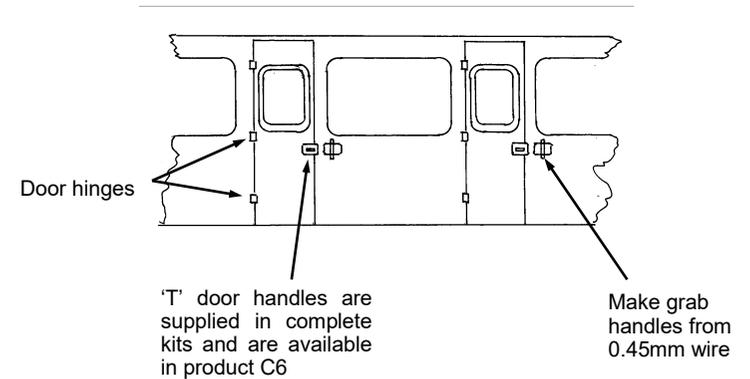
Door hinges, gangway suspension brackets, train alarm gear ears, gangway end covers and solebar ascending steps are available in product C26
