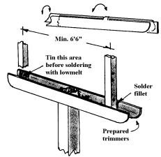
Remove sufficient trimmers from the frets to suit the width of the prototype and split them into linked pairs. Fold each pair back-to-back (halfetched lines on the inside) and sweat together. Remove the resulting "tags". Cut the trimmers to length, and file to the correct end profile (square top corner, round bottom corner).
