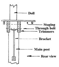
Select the appropriate size and number of brackets (e.g. two small brackets for an equal tee signal). Solder the bracket flanges to the brackets, and the resulting assemblies to the post and trimmers, with the single-holed flange being adjacent to the post. Finally, add the landings; the front should be flush with the trimmer, with the entire overhang thus being at the rear.
