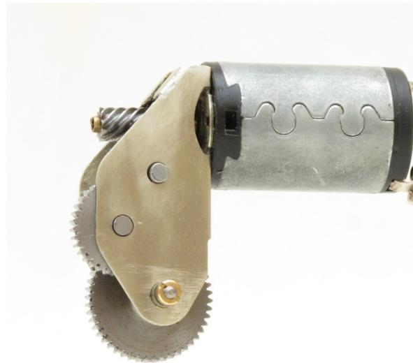
Figure 2 Assembled gearbox and motor
