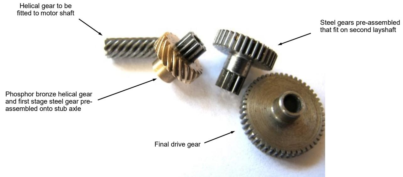
Figure 1 Component gears
