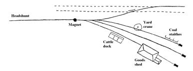
Magnets should be placed at any point where uncoupling is desired, remembering that with the delayed operation feature, wagons can be uncoupled and then pushed as far as needed without recoupling taking place. All the track depicted as a solid line in the example above may be shunted with just the one magnet shown. At pointwork, ensure that the magnet position does not leave wagons within the fouling point of the converging track.
