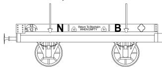
Bodywork, solebars: grey, Precision Paint P679 Buffers, drawgear, running gear and sometimes body ironwork: black
