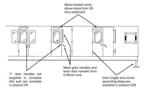
The ends are identical except that the train alarm gear is only fitted at the end shown on the roof plan overleaf
