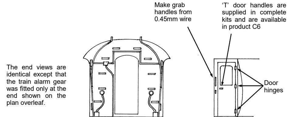
The end views are identical except that the train alarm gear was fitted only at the end shown on the plan overleaf.
