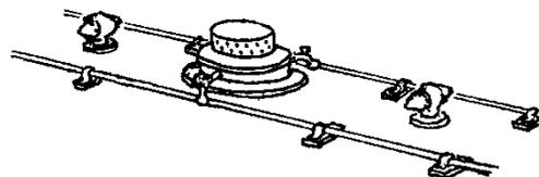
ABOVE - ARRANGEMENT OF PIPING FOR GAS LAMPS, WOODEN MOUNTING BLOCKS AND TORPEDO VENTS.
