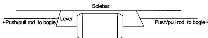
Attach the vacuum cylinder to the centre of the carriage with the lever links pointing at 10° towards the cylinder. Viewed side on, a slight gap should be apparent between the solebar and the cylinder. Attach 0.5mm wire push/pull rods from the lever midpoints towards each bogie.
