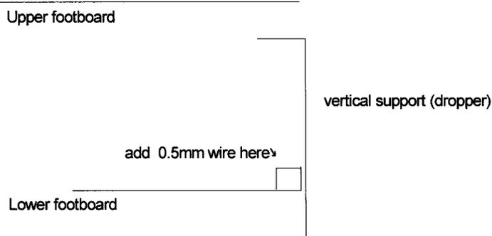
Carefully raise the rivets on the upper footboard (8) attachment tags, then bend them by 90°. Solder a length of 0.5mm wire to the rear edge of each lower footboard (9), on the side without the half-etched indentations. Bend the footboard supports (10) to a U shape and solder them into the indentations on the lower surface of each footboard. The footboard assemblies are now attached to the solebars, working from the tab at one end. The short footplates (11) are not used on this diagram.
