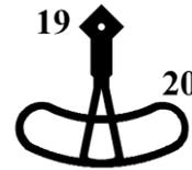
Place the arm spindle into its bearing and ensure it moves freely – clean off any paint that might have crept in. Open out the hole in back-blinder spindle (19) to 0.80mm (no.68). Solder (188°) the spindle to the plain face of back-blinder (20) so the arc on (19) is at the outer edge of (20), and (20) is symmetrical about the axis of (19).
