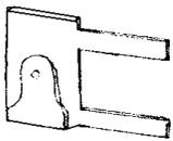
Sweat the two balance weight levers (5) together. Add weights (6) either side to increase the thickness as desired. Open out the
