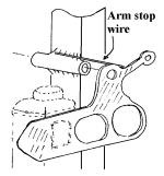
The tube centreline should be 6mm below the post top, and the end should project around 1.5mm in front of the post. Solder  $(70^{\circ})$  the tube to the post. Use the minidrill and slitting disc to trim the rear of the tube so it projects around 1.5mm behind the post. Test fit the arm in the bearing, and trim the stop wire. You may need to file down the top of the spectacle
