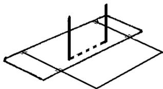
If using the lower mounting height, prepare the coupling loop from MSE's *BW* brass wire.
