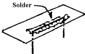
Remove a plate from the fret and burnish both sides. Fold up a wire staple from MSE's *NSW4* nickel silver wire to the shape shown. The legs should be around 6mm long, and 6mm apart for 3mm couplings, or 8mm apart for 4mm couplings.
