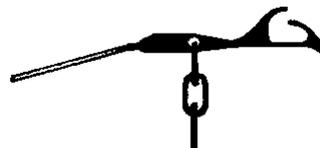
Assemble a 3-link chain as shown, inserting the top link through the dropper hole. Use pliers to close any unsightly gaps.
